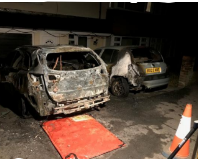
The aftermath of a link box explosion that caused two nearby cars to catch fire
